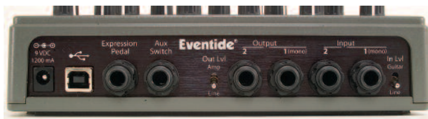
ModFactor's rear panel provides stereo inputs with a Guitar/Line Level switch, stereo outputs with an Amp/Line Level switch, Expression Pedal and Aux Switch jacks, a USB connector for MIDI I/O (standard MIDI In and Out/Thru jacks are located on the side), and a socket for 9VDC/1200mA power.
